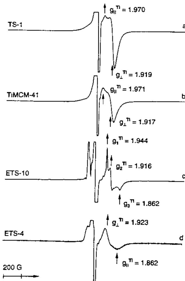
**Fig. 22** ESR spectra at 77 K of (a) TS-1, (b) TiMCM-41, (c) ETS-10, and (d) ETS-4 after  $\gamma$  irradiation at 77 K of activated samples. (From Ref. 28.)
