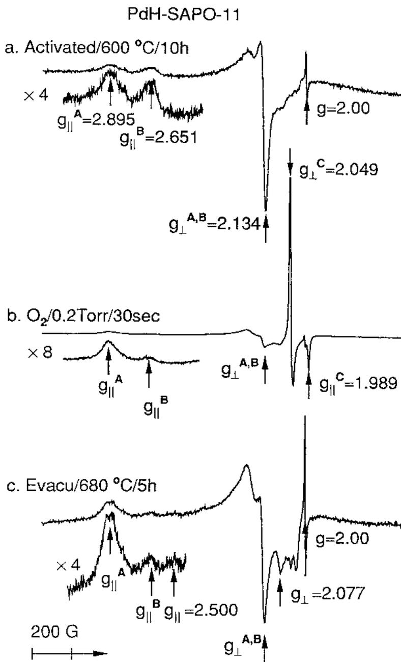
**Fig. 16** ESR spectra at 77 K of (a) PdH-SAPO-11 activated at 600 °C (b) after subsequent adsorption of 0.5 Torr of oxygen at room temperature for 5 min or (c) after further heating at 600 °C for 5 h. (From Ref. 25.)
