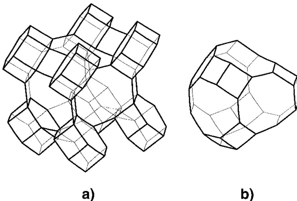
**Fig. 12** SAPO-18 structure (AEI type): (a) hexagonal prisms surrounding the pear-shaped supercage, and (b) the pear-shaped supercage. (From Ref. 24.)
