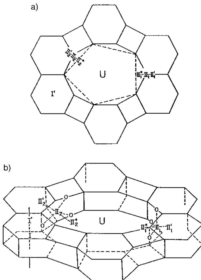
**Fig. 18** (a) View along the elliptical 10-ring channel axis of SAPO-11 where the dashed lines show the edges of six-ring windows that form the surfaces of a 10-ring channel. (b) A simplified structure of SAPO-11 showing possible cation positions. (From Ref. 25.)
