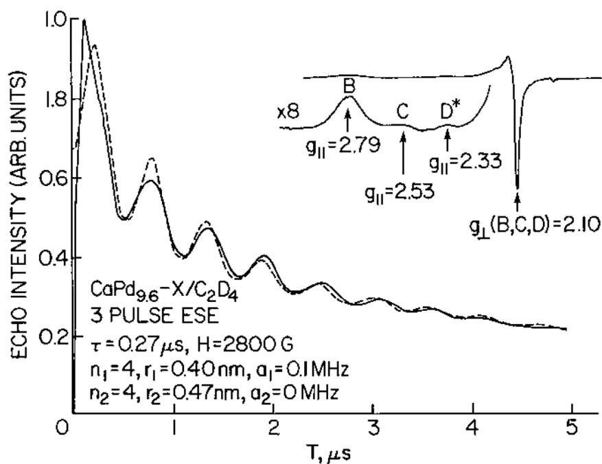
**Fig. 7** Experimental (—) and simulated (----) three-pulse ESEM spectra at 4 K of CaPd<sub>9.6</sub>-X with adsorbed C<sub>2</sub>D<sub>4</sub> at  $g_{||} = 2.33$  as indicated by an asterisk on the inset ESR spectrum at 77 K. (From Ref. 22.)
