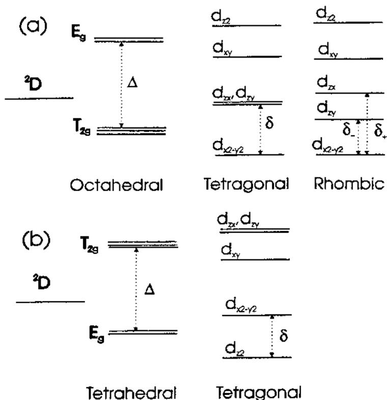
**Fig. 23** Energy levels of a  $3d^1$  ion in (a) octahedral and (b) tetrahedral cubic fields. (From Ref. 28.)
