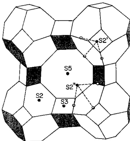
**Fig. 1** Crystal structure of zeolite A showing cation positions. Site S2 is at the center of a six-ring face with site S2' and S2\* displaced into and out of the β cage along the triad axis, respectively. Site S3 is adjacent to the 4-ring in the α cage while site S5 is at the center of the octagonal window. (From Ref. 17.)
