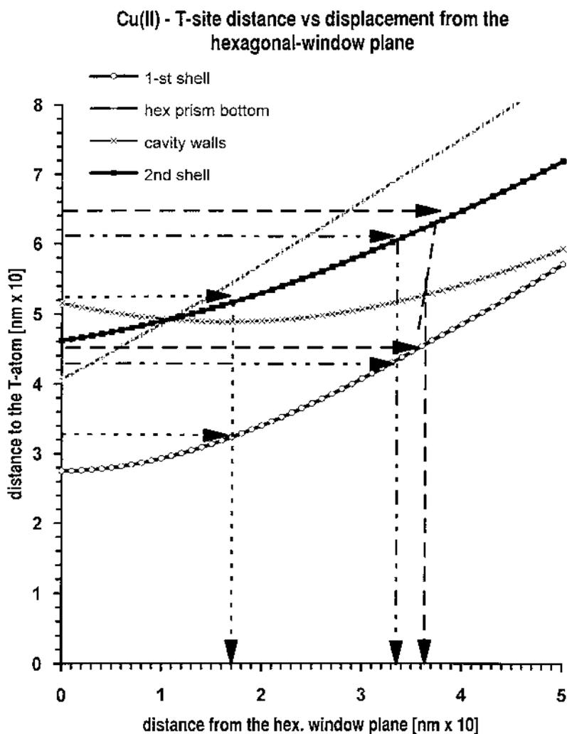
**Fig. 14** Displacement of  $\text{Cu}^{2+}$  ion from the plane of the hexagonal ring in the supercage of Cu-SAPO-18 from three pulse  $^{31}\text{P}$  ESEM simulations. The second shell curve (solid squares) is an average of the curves for the distances to the bottom of the hexagonal prism (+) and the distances to T sites located on the wall of the cavity (x). (From Ref. 24.)
