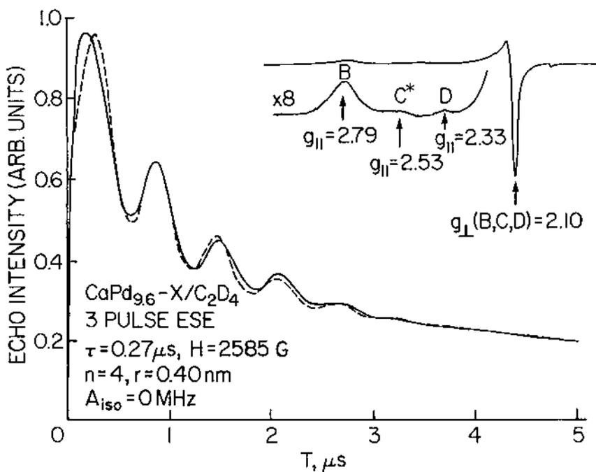
**Fig. 6** Experimental (—) and simulated (----) three-pulse ESEM spectra at 4 K of NaPd<sub>12.5</sub>-X with adsorbed C<sub>2</sub>D<sub>4</sub> at 50°C at  $g_{\parallel} = 2.53$  indicated by an asterisk inset ESR spectrum at 77 K. (From Ref. 22.)
