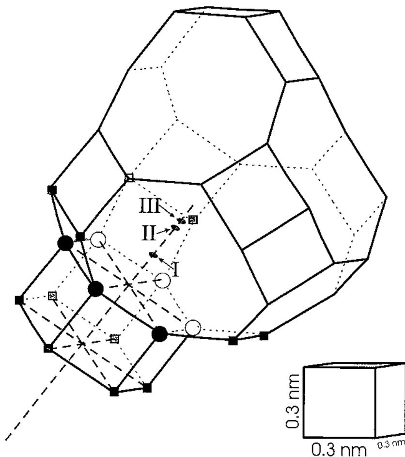
**Fig. 15** Schematic of first (circles) and second (squares) shell T-site positions around  $\text{Cu}^{2+}$  in Cu-SAPO-18 from three-pulse  $^{31}\text{P}$  ESEM data and the  $\text{Cu}^{2+}$  positions in (I) Cu-SAPO-18 dehydrated at  $400^\circ\text{C}$  overnight, (II) Cu-SAPO-18 rehydrated at  $100^\circ\text{C}$  overnight, and (III) fresh Cu-SAPO-18 after ion exchange. (From Ref. 24.)
