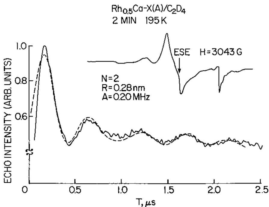
**Fig. 10** Three-pulse ESEM spectrum with corresponding ESR spectrum of Rh<sub>0.5</sub>Ca-X (A) followed by C<sub>2</sub>D<sub>4</sub> adsorption at 77 K and warming to 195 K for 2 min. The ESEM was measured at  $H = 3043$  G with  $\tau = 0.30$   $\mu$ s. The dashed trace is a calculated spectrum, and the corresponding best-fit parameters are shown. (From Ref. 23.)
