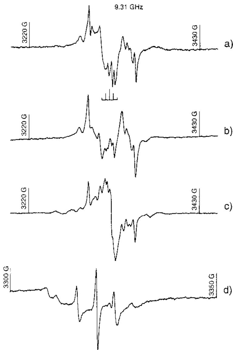
**Fig. 26** ESR spectra obtained at 70 K after 77 K  $\gamma$  irradiation of (a) Na-ZSM-5(Si/Al = 1000), (b) Na-ZSM-5(Si/Al = 170), and (c) Na-ZSM-5(Si/Al = 40) containing 0.1% acetylene. Part (d) shows the ESR spectrum obtained at 130 K after 77 K  $\gamma$  irradiation of Na-ZSM-5(Si/Al = 40) containing 0.1% acetylene. (From Ref. 34.)
