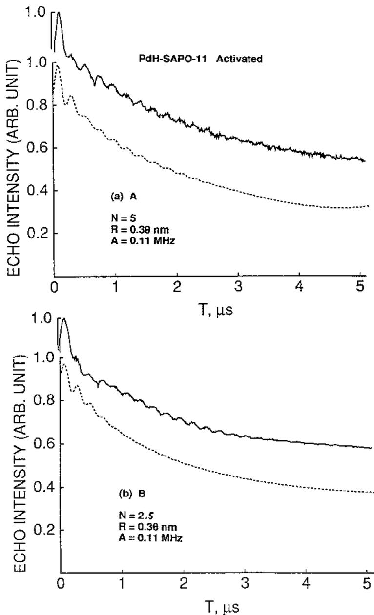
**Fig. 17** Experimental (—) and simulated (----) three-pulse ESEM spectra at 4 K of activated PdH-SAPO-11 at the magnetic field corresponding to (a) the  $g_{\parallel}$  value of  $\text{Pd}^+$  species A and (b) the  $g_{\parallel}$  value of  $\text{Pd}^+$  species B showing  $^{31}\text{P}$  modulation. (From Ref. 25.)
