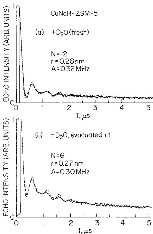
**Fig. 4** Experimental (—) and simulated (----) three-pulse ESEM spectra recorded at 4 K of CuNaH-ZSM-5 (a) with adsorbed D<sub>2</sub>O and (b) with adsorbed D<sub>2</sub>O followed by evacuation at room temperature. (From Ref. 20.)
