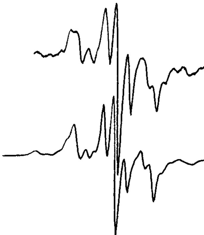
**Fig. 24** Comparison of experimental (upper) and simulated (lower) powder ESR spectra of the naphthalene- $h_8$  radical cation at 77 K in H-ZSM-5 zeolite. (From Ref. 33.)
