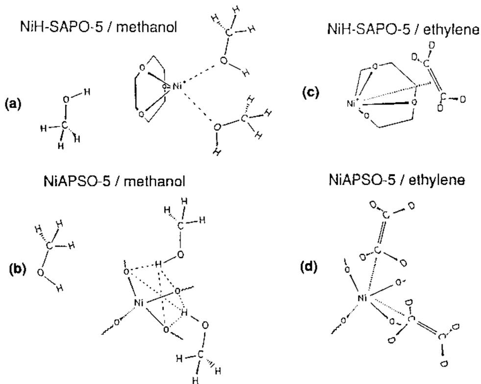
**Fig. 21** Schematic diagram of  $\text{Ni}^+$  coordinated to methanol in (a) NiH-SAPO-5 and (b) NiAPSO-5 and to ethylene in (c) NiH-SAPO-5 and (d) NiAPSO-5. (From Ref. 26.)
