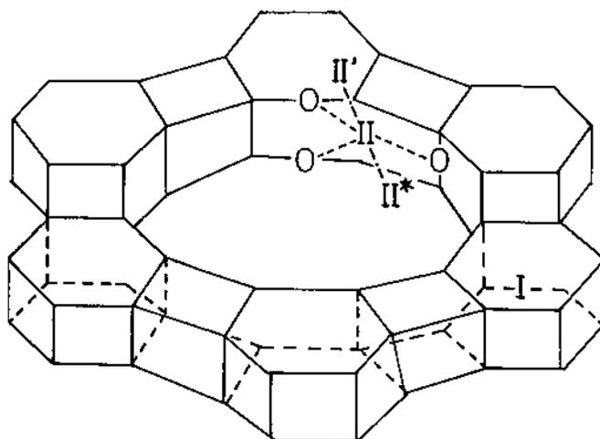
Fig. 19 SAPO-5 structure showing possible cation positions.
