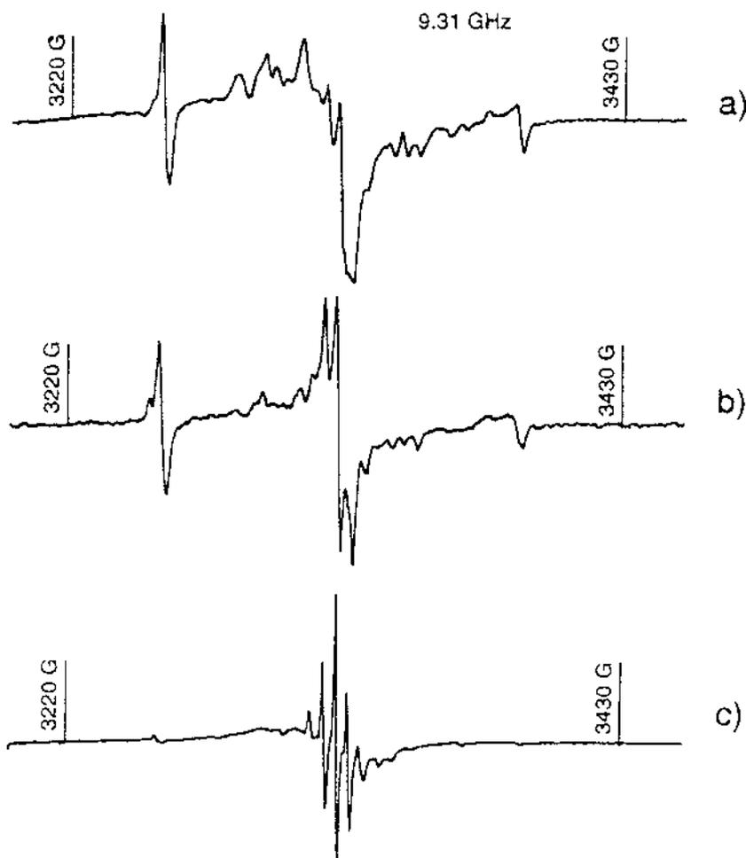
**Fig. 25** ESR spectra obtained at 70 K after 77 K  $\gamma$  irradiation of (a) H-ZSM-5(Si/Al = 400), (b) H-ZSM-5(Si/Al = 240), and (c) H-ZSM-5(Si/Al = 50) containing 0.1% acetylene. (From Ref. 34.)
