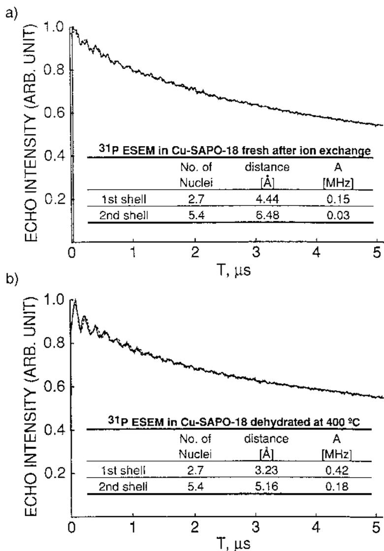
**Fig. 13** Three-pulse  $^{31}\text{P}$  ESEM at 5 K (solid line) and simulation (dashed line) for (a) fresh Cu-SAPO-18 after ion exchange and (b) Cu-SAPO-18 dehydrated at 400 °C overnight. (From Ref. 24.)
