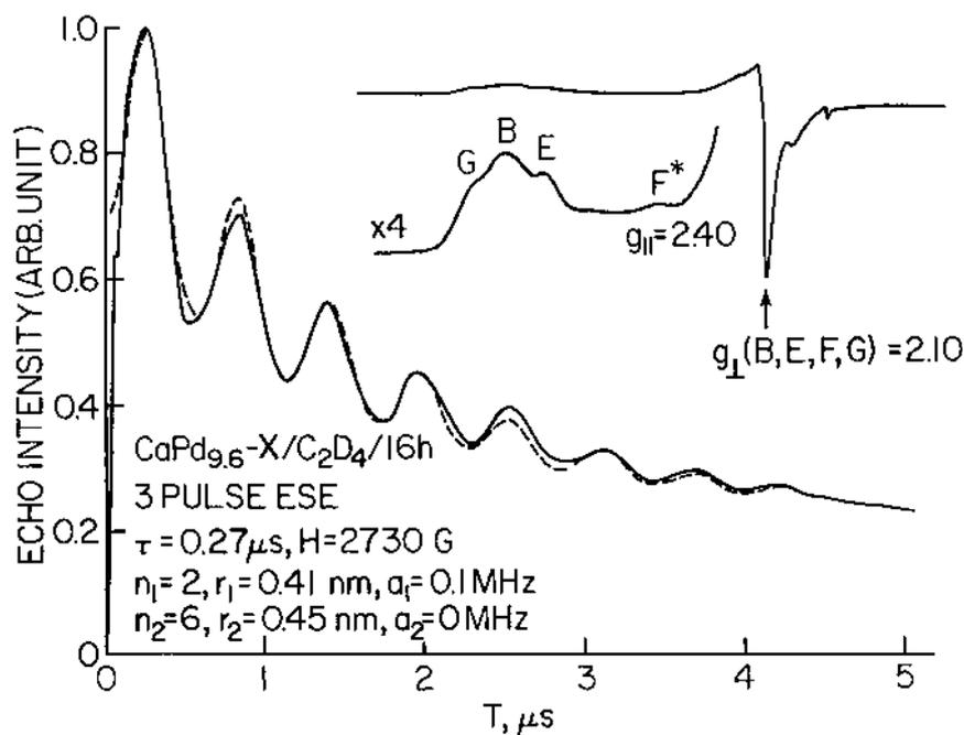
**Fig. 8** Experimental (—) and simulated (----) three-pulse ESEM spectra at 4 K of CaPd<sub>9.6</sub>-X with adsorbed C<sub>2</sub>D<sub>4</sub> at  $g_{||} = 2.40$  as indicated by an asterisk on the inset ESR spectrum at 77 K. (From Ref. 22.)
