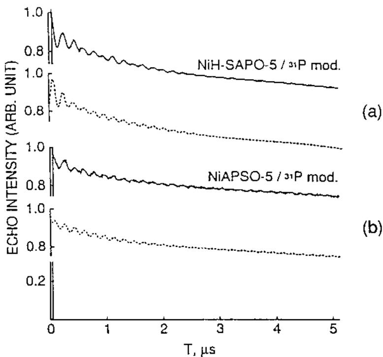
Fig. 20 Experimental (—) and simulated (----) three-pulse ESEM spectra showing  $^{31}\text{P}$  modulation for (a) NiH-SAPO-5 and (b) NiAPSO-5 after hydrogen reduction and subsequent 10-min evacuation at room temperature. Spectra recorded at 4 K with  $\tau = 0.27 \mu\text{s}$  to suppress  $^{27}\text{Al}$  modulation. (From Ref. 26.)
