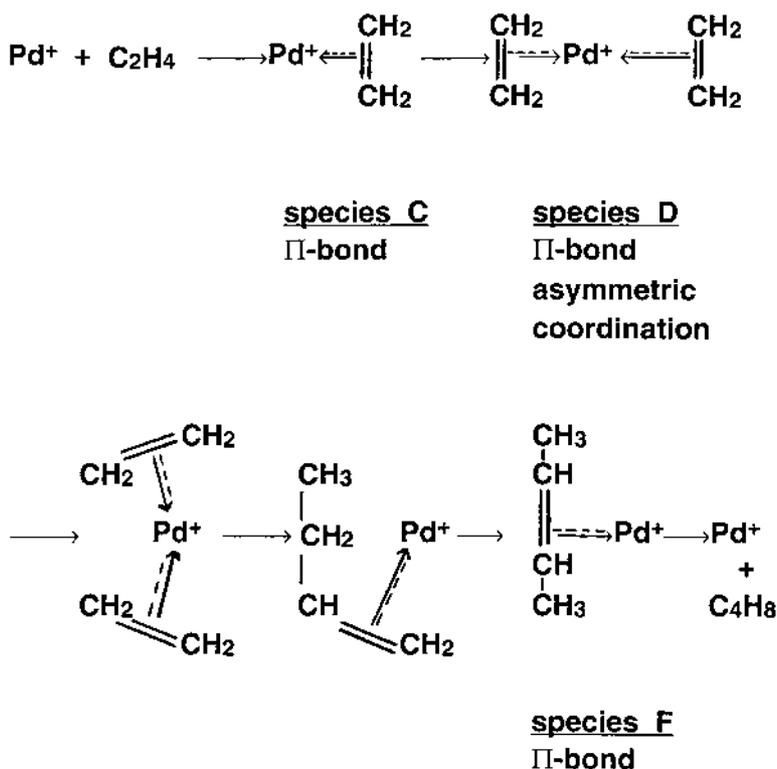
Fig. 9 Pd<sup>+</sup>-catalyzed ethylene dimerization mechanism on PdCa-X zeolite.
