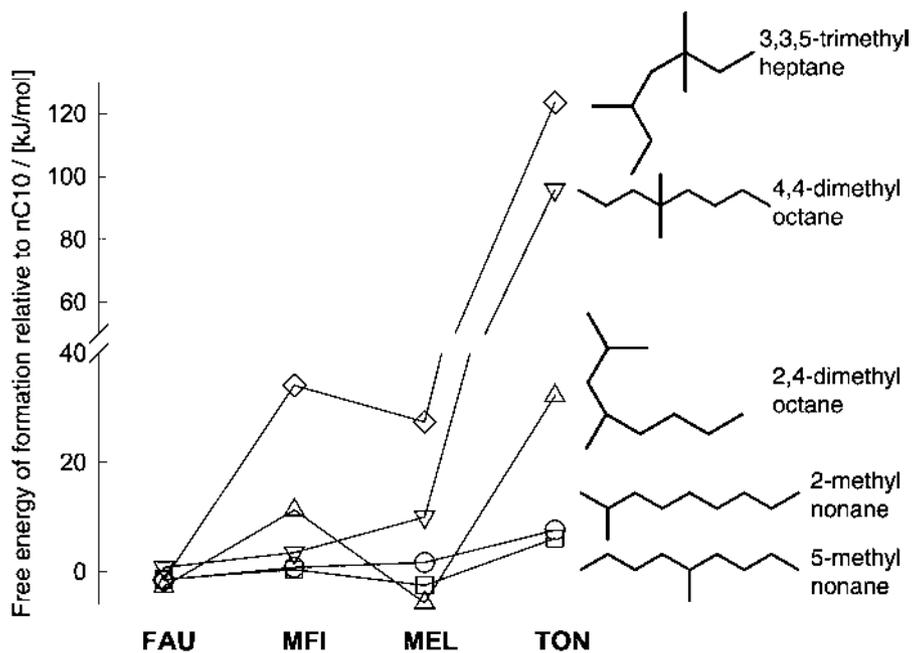
**Fig. 18** The Gibbs free energy of formation of 2-methylnonane, 5-methylnonane, 2,4-dimethyloctane, 4,4-dimethyloctane, and 3,3,5-trimethylheptane, relative to *n*-decane in the zeolites FAU, TON, MFI, and MEL. Calculations from CBMC simulations (Refs. 44 and 45).
