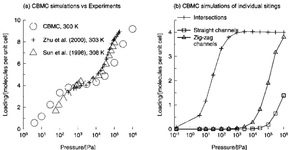
**Fig. 5** (a) Comparison of experimental data (Refs. 25,26) for pure component isotherm for isobutane in MFI at 300 K with CBMC simulations (Refs. 23,24). (b) Loadings of isobutane at 300 K in intersection sites, straight channels, and zig-zag channels. The cutoff radius of sphere defining the intersection site is 0.3 nm. Simulation results from Ref. 24.
