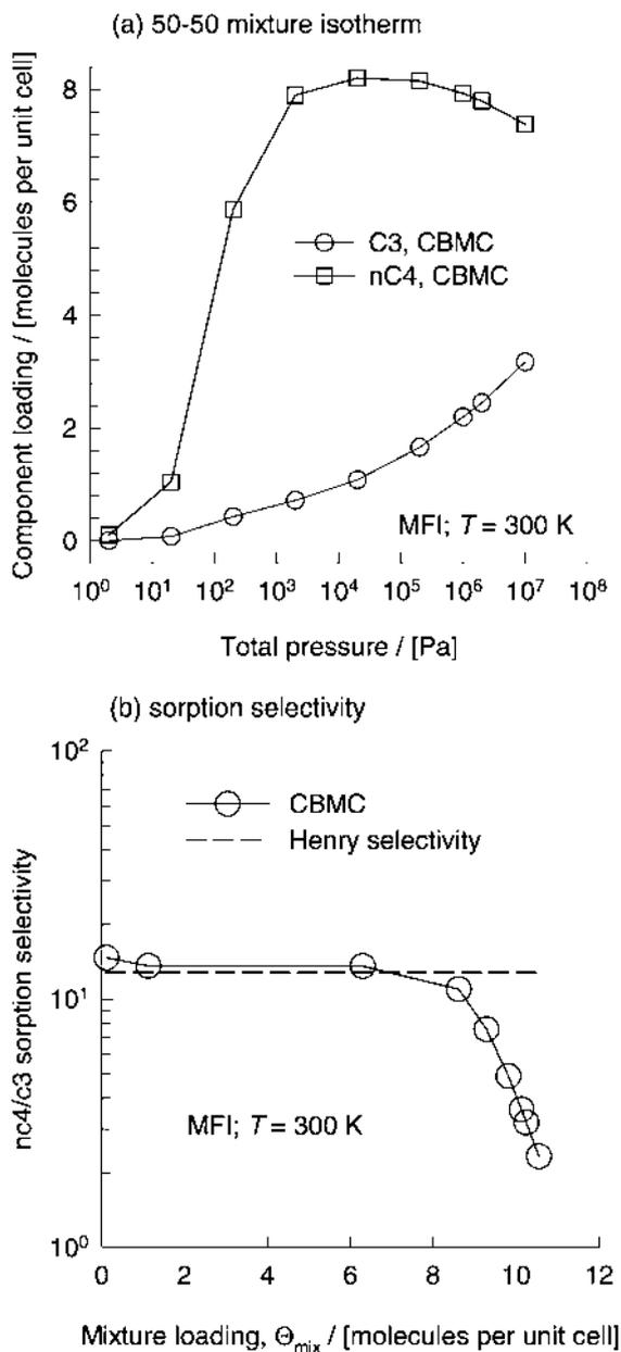
**Fig. 12** (a) Adsorption loadings of equimolar binary mixture of C3 and nC4. (b) nC4/C3 adsorption selectivity.
