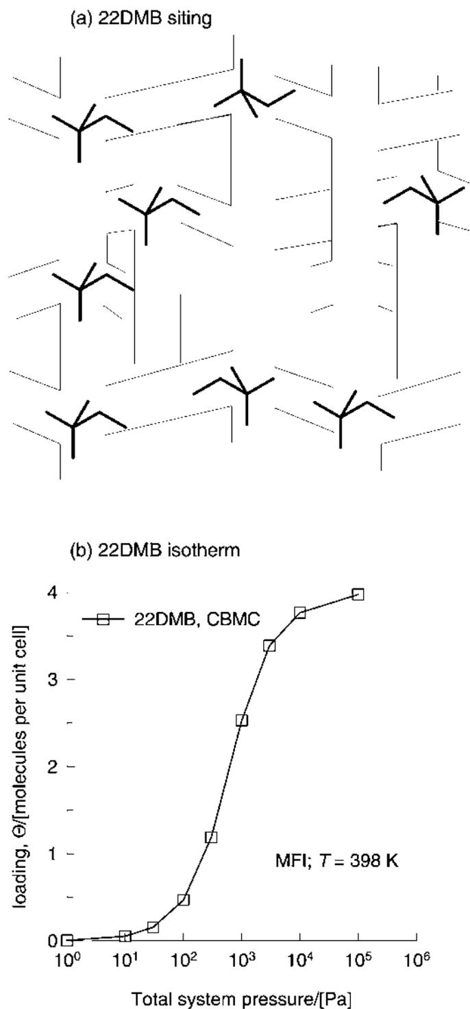
**Fig. 8** (a) Schematic showing preferential location of 2,2-dimethylbutane (22DMB) at intersections between straight and zig-zag channels of MFI network. (b) CBMC simulations of pure component isotherm for 22DMB in MFI at 398 K.
