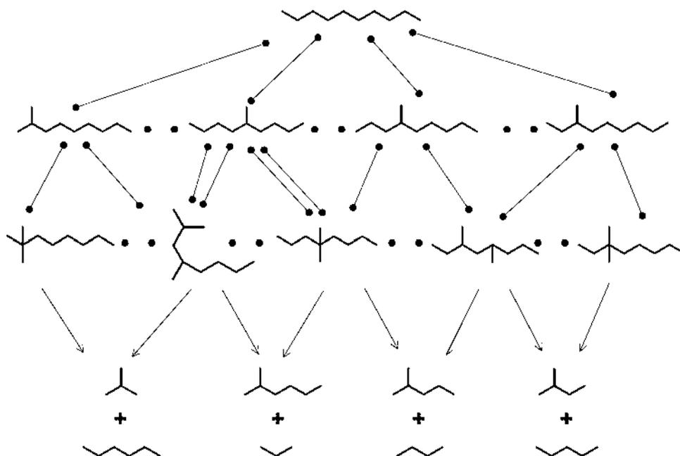
**Fig. 17** Reaction pathways during hydrocracking of *n*-C10. Equilibration between isomers is denoted by lines with black dots at either end. Hydrocracking is denoted by arrows. As the methyl nonanes can hydroisomerize into 2,4-dimethyloctane and 4,4-dimethyloctane by three different routes, these two methyloctanes are kinetically favored. This is the simplified reaction scheme adapted from Maesen et al. (44).
