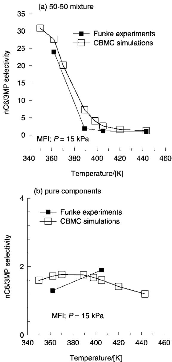
**Fig. 14** (a) Adsorption selectivities calculated by CBMC simulations of 50:50 mixture of nC6–3MP at various temperatures in MFI, keeping the total pressure at 15 kPa. (b) Adsorption selectivities based on pure component loadings at various temperatures, keeping the total pressure at 15 kPa. Also shown are the experimentally determined membrane permeation selectivities of Funke et al. (Ref. 40).
