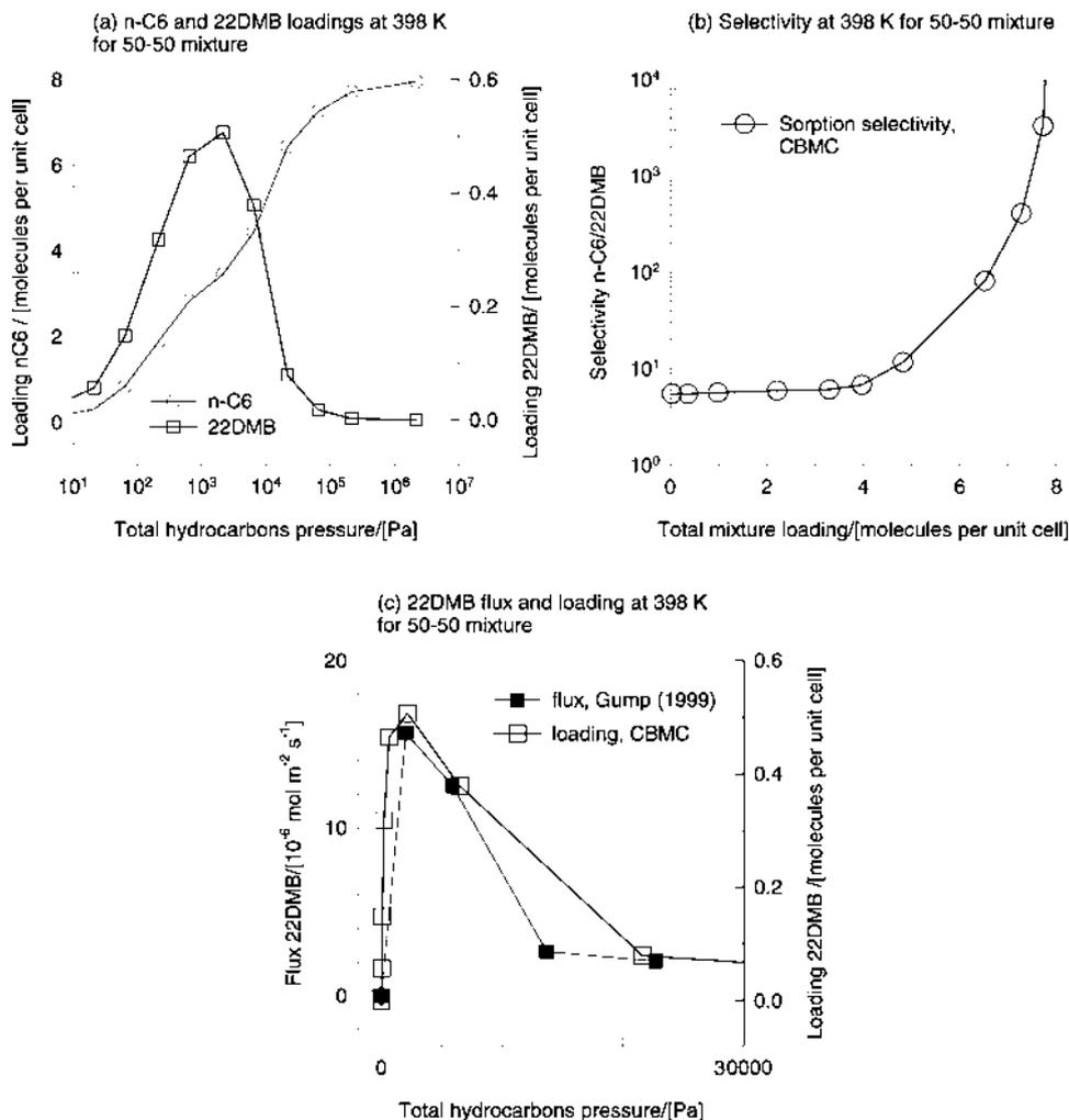
**Fig. 15** (a) CBMC simulations of 50:50 mixture isotherm for nC6–22DMB at 398 K in MFI. (b) Adsorption selectivity as a function of total mixture loadings. (c) Comparison of loading of 22DMB with fluxes measured by Gump et al. (Ref. 41).
