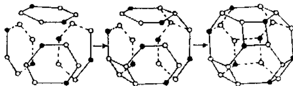
Fig. 32 Scheme for the formation of nuclei of zeolite Y. (From Ref. 22.)
